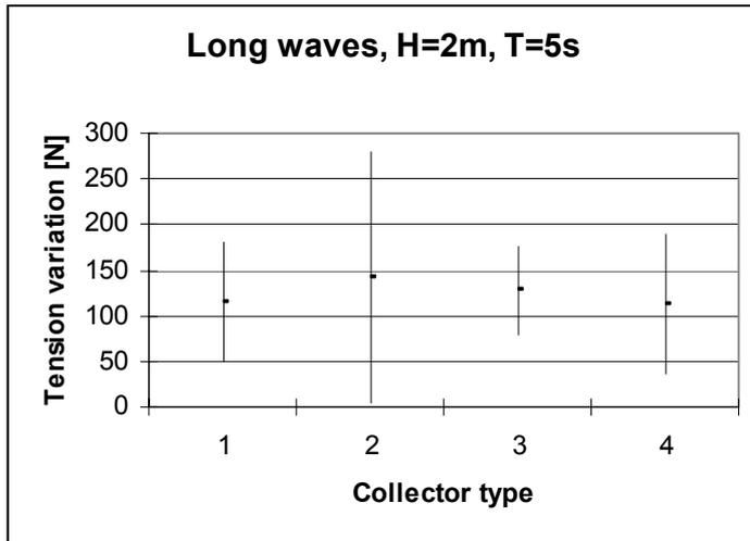
**Figure 5.** This wave condition represents long waves with a wave height/ wavelength ratio of 1/18
