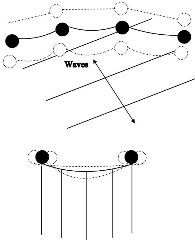
**Figure 6.** Illustrates how large horizontal deflection from long waves causes the hanging span between the buoys to stretch. This causes large accelerations on the collectors.
