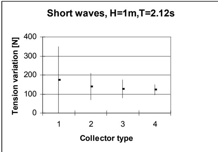
**Figure 3.** Tension variation in collectors for short, steep waves.
