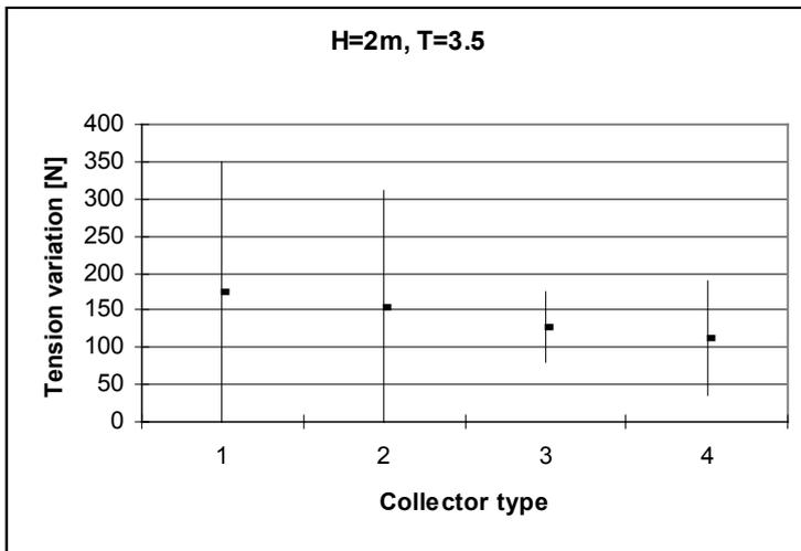
**Figure 4.** Larger waves causes snap loads for the longline system, while the longtube motions are still acceptable.
