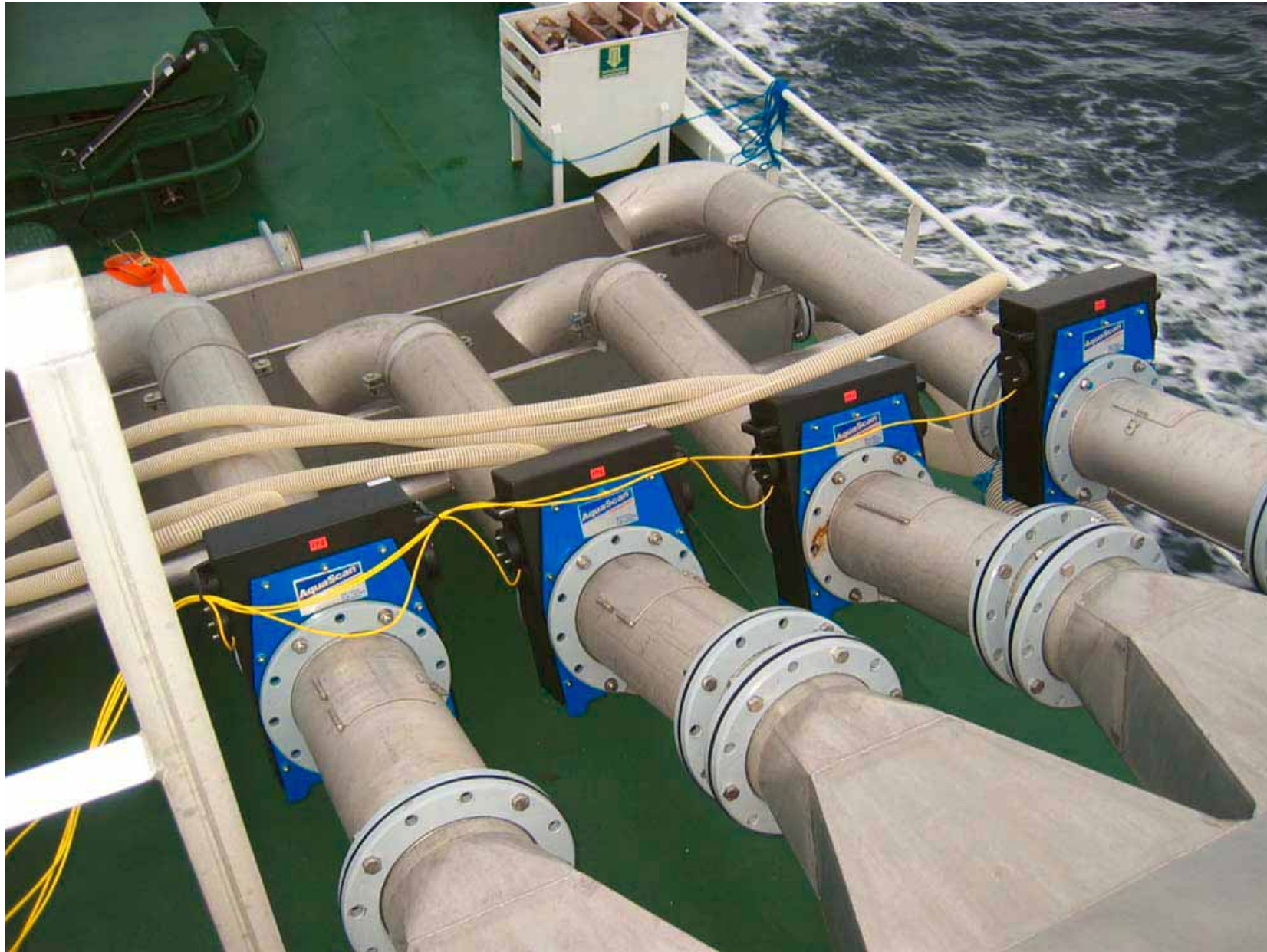
Reg. Units CSE3150 (12") connected to a grader at a well boat. Same way of operation as with CSE1600 (6")
