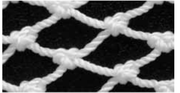
Fig. 8: Picture of a traditional mesh with knots. Twine diameter d = 1.2 [mm] and halfmesh opening \lambda = 10.0 [mm] .
